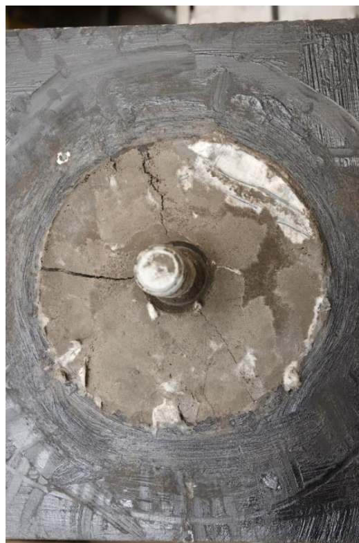
Figure 20 Paper package soaking time effect on grout penetration under the dome-plate at: a) 10 minutes, b) 12 minutes, c) 15 minutes and d) 20 minutes
