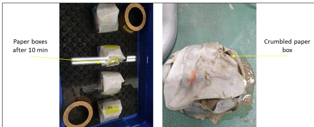
Figure 3 Condition of paper boxes after 10 min submerged in water.
