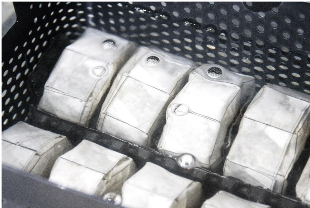
Figure 29. Package with pucks immersed in water (a) escaping air bubbles (b).
