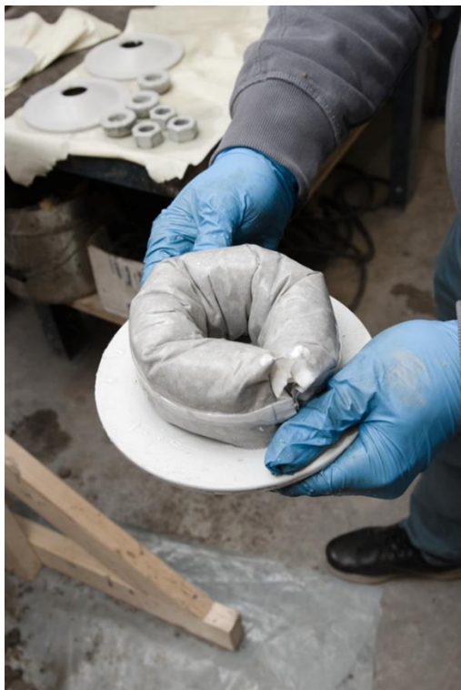
Figure 22 a) Doughnut shape package and b) even grout distribution under the plate with paper concentration area
