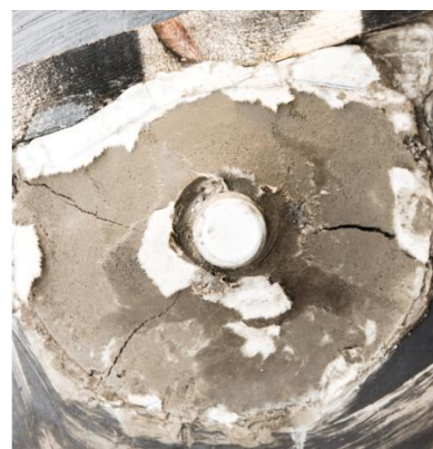
Figure 21 Uneven surface effect on grout distribution under the dome-plate: a) 12 minutes paper package soaking time and 12mm obstacle; b) 12 minutes paper package soaking time, 20 mm obstacle and sealed edged with the grease to prevent evaporation of water during grout hardening; c) 12 minutes paper package soaking time, 20 mm obstacle without sealed edges
