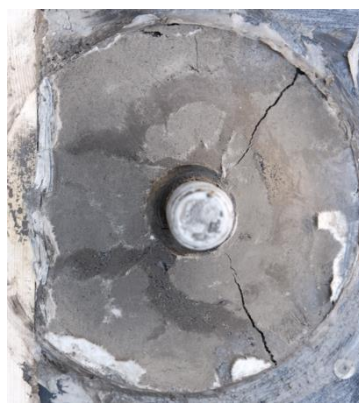
Figure 21 Uneven surface effect on grout distribution under the dome-plate: a) 12 minutes paper package soaking time and 12mm obstacle; b) 12 minutes paper package soaking time, 20 mm obstacle and sealed edged with the grease to prevent evaporation of water during grout hardening; c) 12 minutes paper package soaking time, 20 mm obstacle without sealed edges
