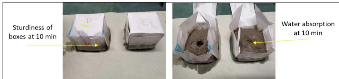
Figure 4 Water absorption and condition of boxes after 10 min.
