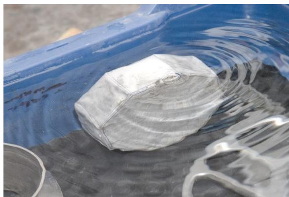
Figure 18 a) Paper package improvement by using second box instead of the lid, b) puncturing the package for better bursting towards borehole, c) putting the package to the water in vertical direction so that the air be able to escape through the joints
