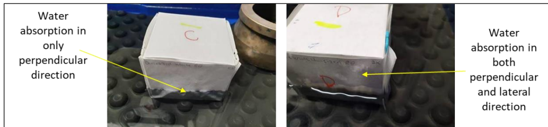
Figure 5 Direction of water absorption in the paper C and D boxes.
