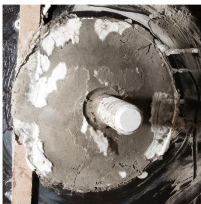
Figure 21 Uneven surface effect on grout distribution under the dome-plate: a) 12 minutes paper package soaking time and 12mm obstacle; b) 12 minutes paper package soaking time, 20 mm obstacle and sealed edged with the grease to prevent evaporation of water during grout hardening; c) 12 minutes paper package soaking time, 20 mm obstacle without sealed edges
